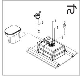
Always use reinforced and odour-tight waste water hoses. Avoid sharp bends or kinks. Connect the toilet to the ø38mm hose connector to the side of the tank. Connect the discharge hose to the ø 38 mm connector onto the tank cover.
