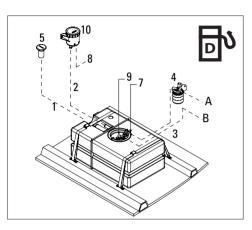
Install the tank in a well-ventilated space on board. Only use fuel resisting hoses and avoid sharp bends and kinks. Make sure that the hoses are not resting on sharp edges, so as to avoid chafing. The ø38mm fuel filling hose must be connected to the corresponding stub on the tank. The suction line (A) and the return line (B) are to be connected to the corresponding connectors on top of the inspection cover.
